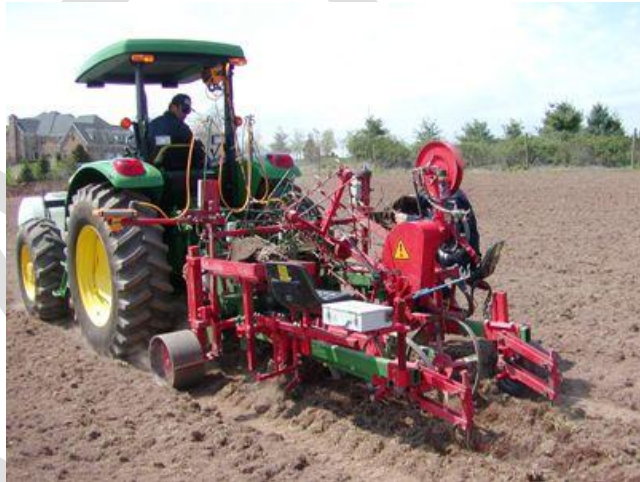
A laser planter gives straight rows in all directions
